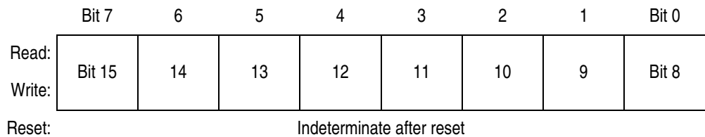
Figure 11-12. TIM Channel 0 Register High (TCH0H)
