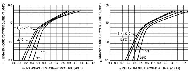
Figure 1. Typical Forward Voltage
