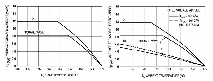
Figure 5. Current Derating, Case Per Leg
