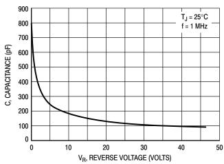
Figure 8. Typical Capacitance
