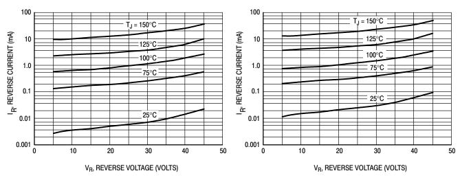
**Figure 3. Typical Reverse Current**
