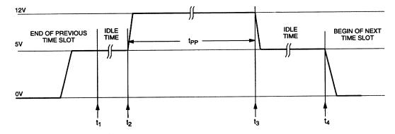
A correct programming pulse can only be generated if the 12V programming voltage is available at the  $V_{PP}$  pin of the DS2480B. The rising and falling edges of the programming pulse are actively controlled by DS2480B. The slew rate is approximately  $14V/\mu s$  and meets the requirements of 1-Wire EPROM devices.
