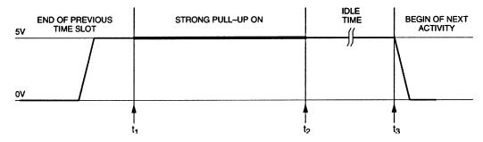
For infinite duration (Figure 9b) the strong pullup also begins immediately after the time slot is completed. To end the strong pullup, the DS2480B must receive a Termination command, code F1h, which occurs at t<sub>2</sub>. The termination command does not generate a response byte. The DS2480B will then immediately end the strong pullup and send out a pulse response byte. Everything else is the same as with predefined duration.
