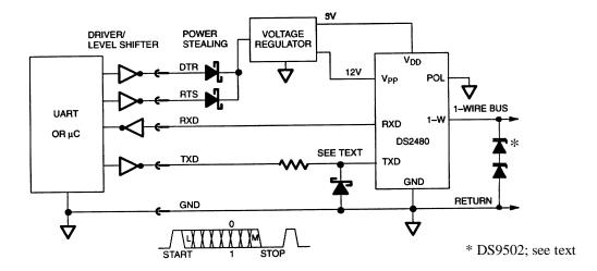
The signals DTR and RTS provide the power to operate the DS2480B. The resistor in the TXD line and the Schottky diode limit the negative voltage at the TXD pin of the DS2480B to 0.3V maximum. The resistor is typically 4.7 k $\Omega$ . If the inverting driver is current–limited to 1 mA the resistor is not required.
