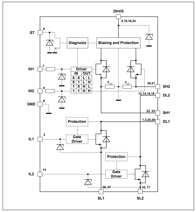
Figure 2 Block Diagram
